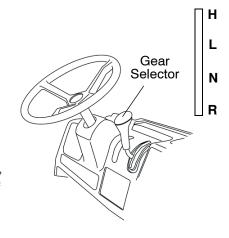
**NOTE:** Maintaining shift linkage adjustment is important to assure proper transmission function. See your dealer if you experience any shifting problems.
